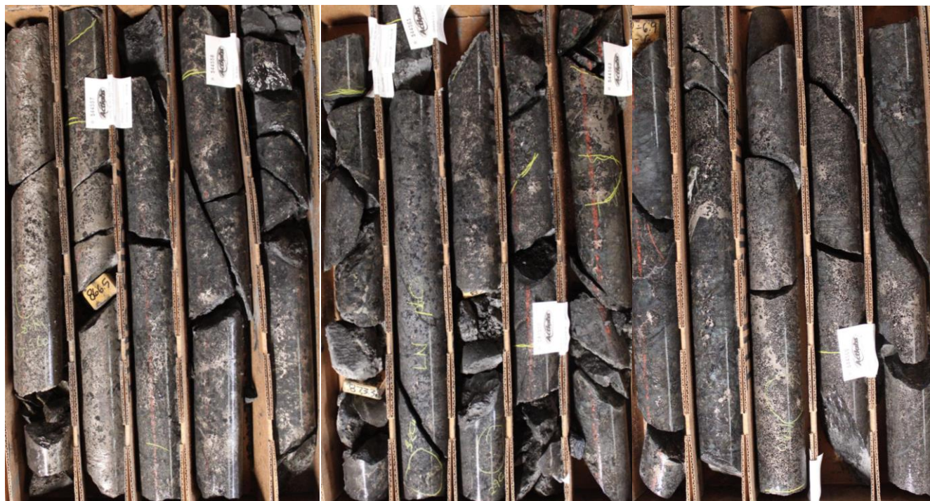
Figure 1 - Significant sulphide mineralization in hole CM2023-06 from approximately 865 to 888 feet (263.7 to 270.7 meters) depth as part of a broader mineralized interval from approximately 841 to 919 feet (256.4 to 280.1 meters) depth which tested a large and previously untested geophysical anomaly.
